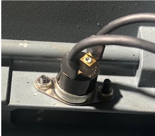
Fig.15 Temperature sensor secured to motor
