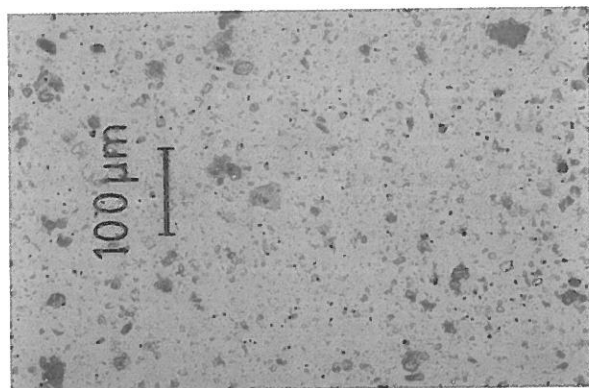
Figures 3 and 4 Photomicrographs of dispersion sample 2/2693. Photographed at plane polarised light at 250x magnification. Sample 2/2693 from Tamassos Cyprus, was found to be composed of three distinct phases, each of which is associated with the manufacture of Egyptian blue. These were Egyptian blue crystals, glass, and residual quartz. In plane polarised light, the particles of the first phase displayed angular habit and a bluish colour; on rotation of the stage they showed moderate pleochroism [Figures 1 and 2]. In crossed polars they were birefringent with high order interference colours. [Photomicrographs: Kakoulli 1999]
