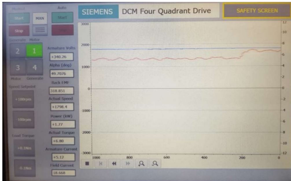
Figure 12 practical continuous current test 3 HMI
