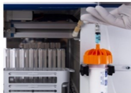
10G Open Cap attached to the Biotage Sfar 10G Column & a Column being filled through the Luer port.
