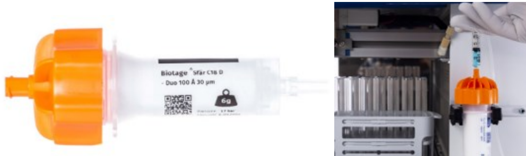
Figure 2 - Biotage Sfär Column & Liquid loading through Luer port
