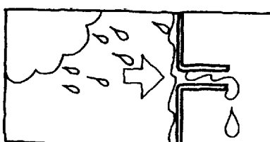
Figure F2.12 Air pressure differentials
