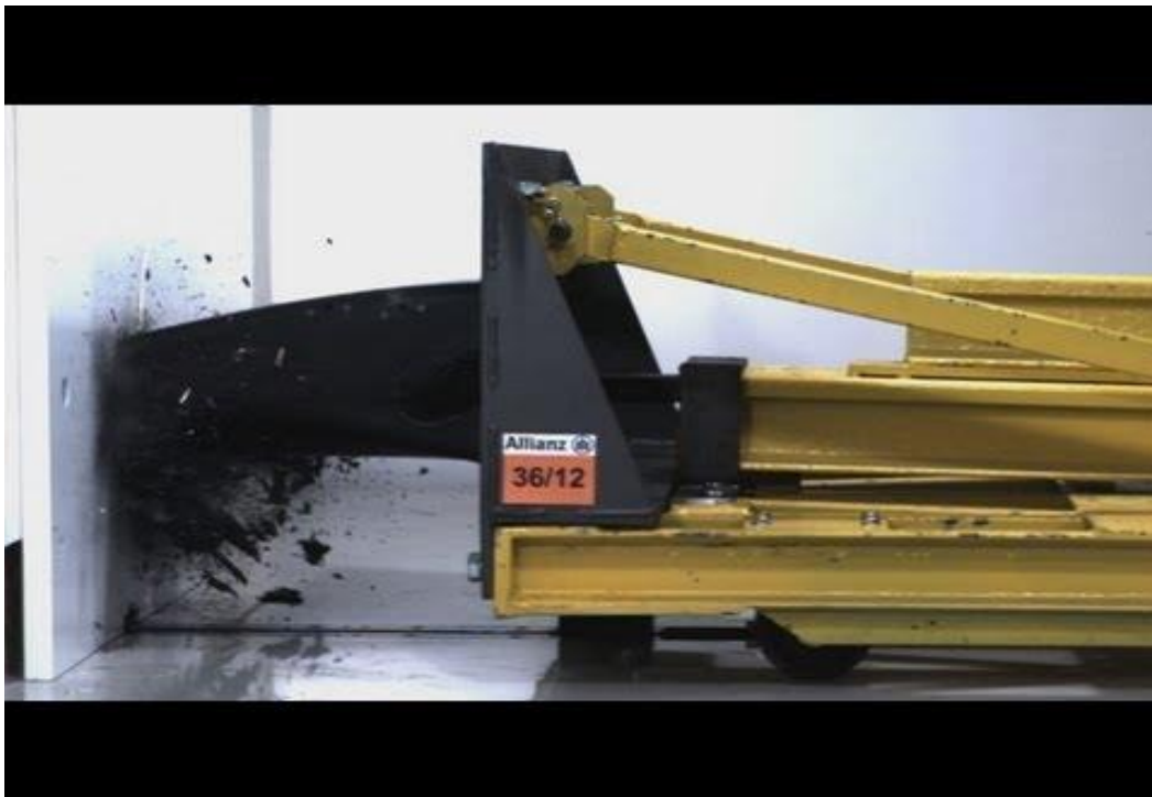
Figure 8-Example of Monocoque Crash Testing (Grand Prix Insights- Monocoque (Including Spectacular Crash Test), 2012)
