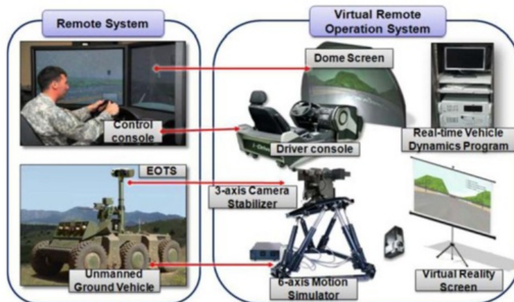
Figure 16 Concept of the indoor remote operating system
