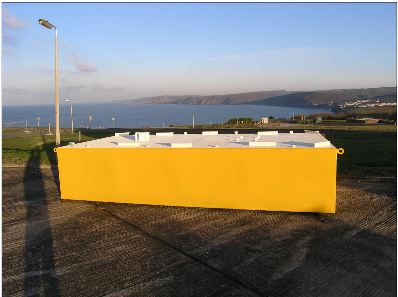
Figure 8 - Manufactured 5 metre pontoon at Aberporth
