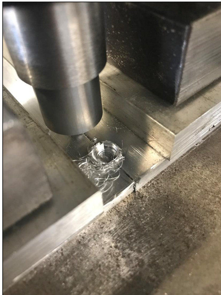
Figure 38 - Tool pin failure during plunge
