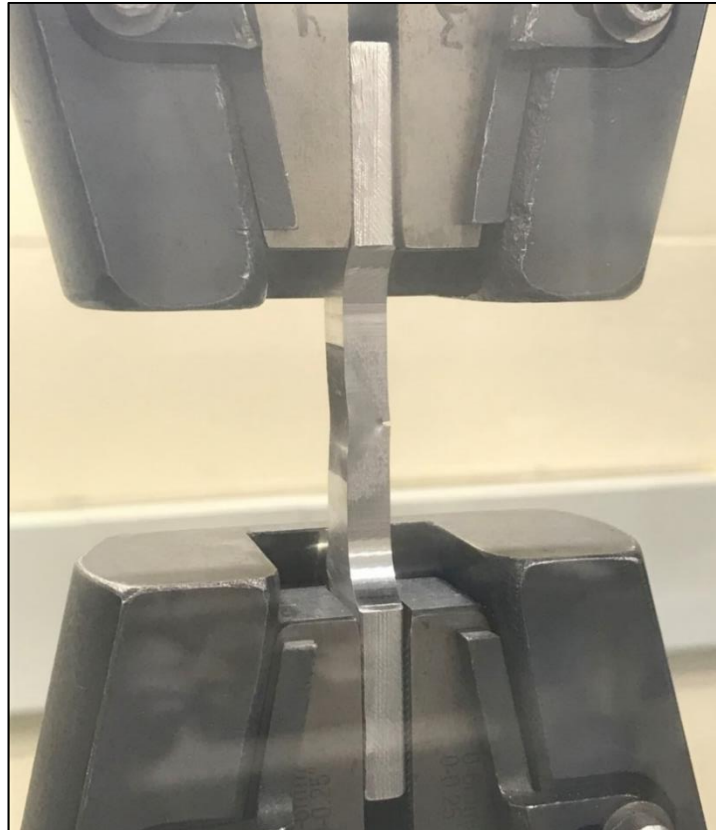
Figure 47 - Loaded tensile sample
