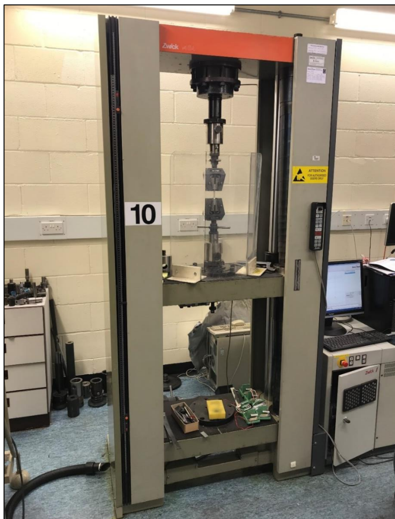
Figure 39 - Zwick/Roell 200kN UTM
