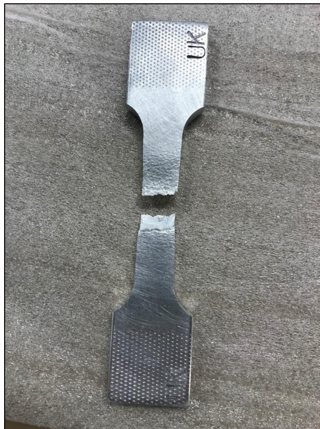
Figure 48 - Pulled sample UK
