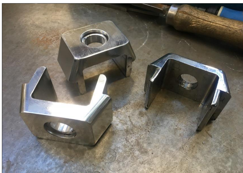
Figure 2 - Welded and machined safety brackets
