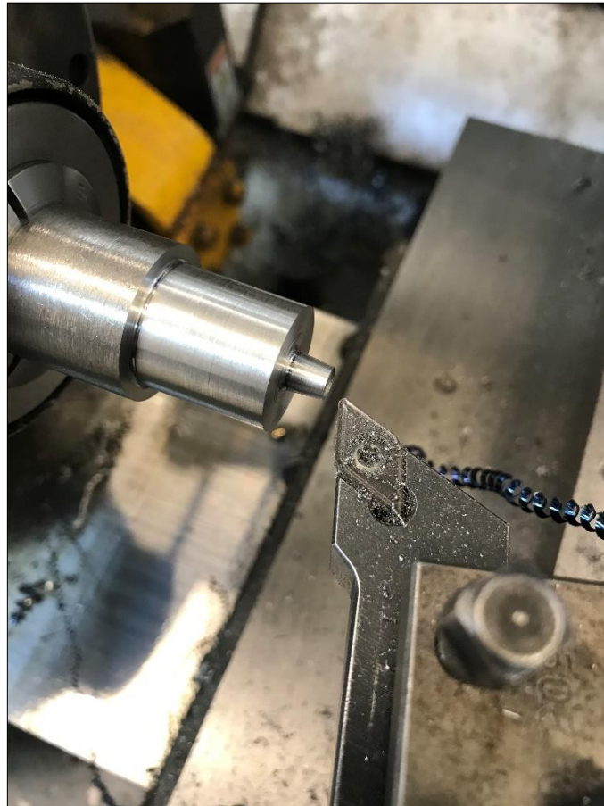
Figure 24 - Tapered tool pin manufacture
