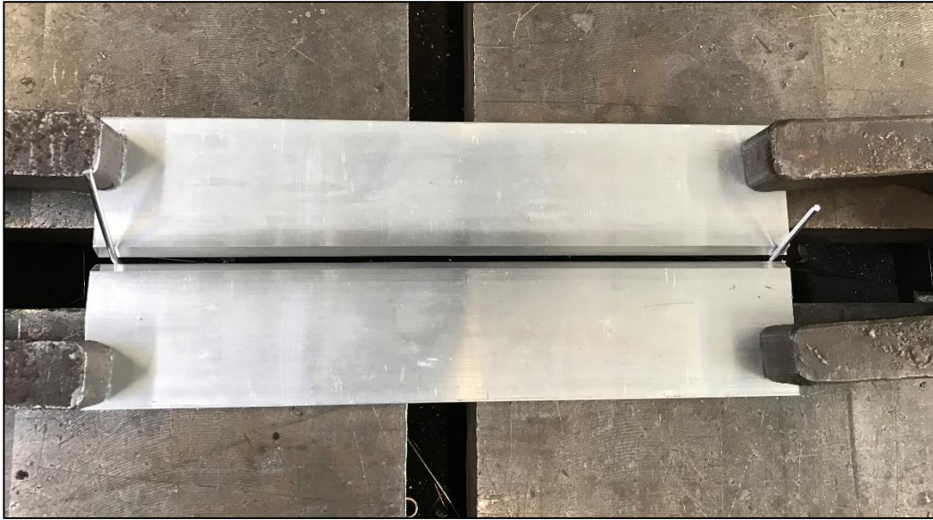
Figure 37 - Conventional weld setup
