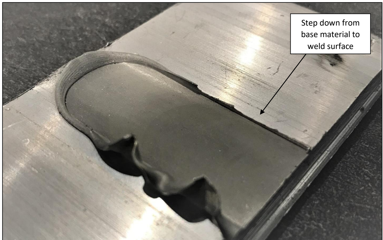
Figure 33 - Deep tool depth
