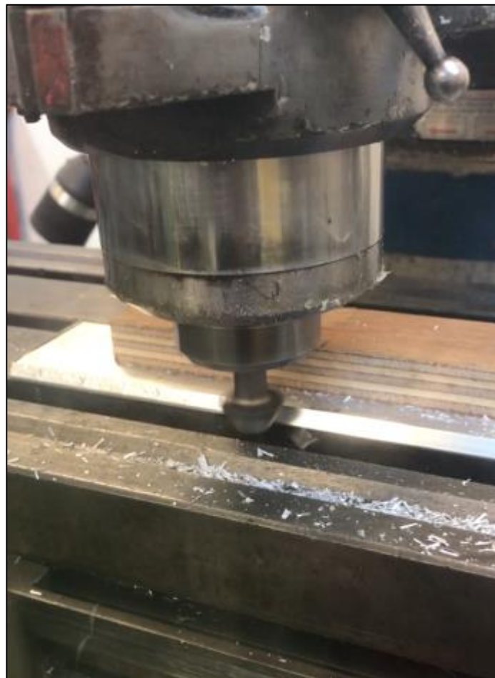
Figure 36 - Sample edge preparation
