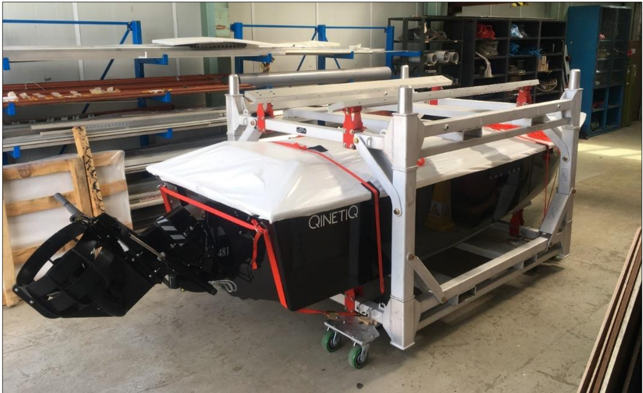
Figure 3 - Unmanned target transport system
