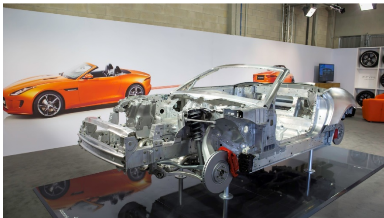
Figure 12: Jaguar F-Type 2014 Chassis (Ireson, 2013.)
