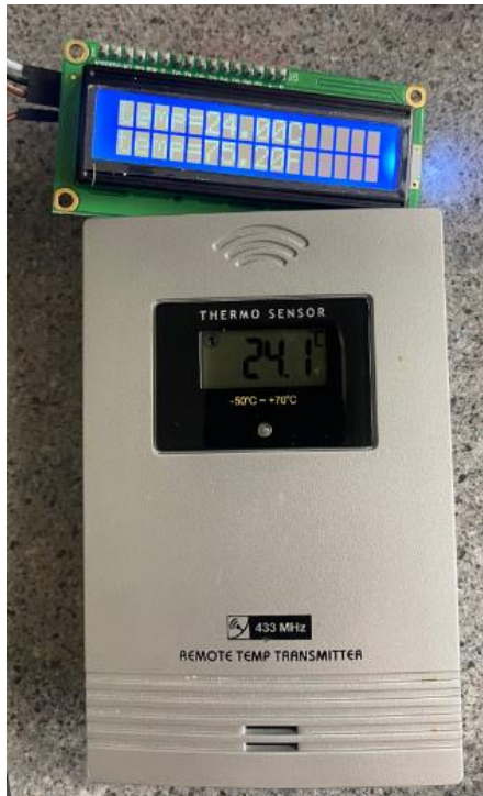
Figure 4- Comparing LCD temperature reading with a calibrated thermo sensor Accessed on 05/05/2023.
