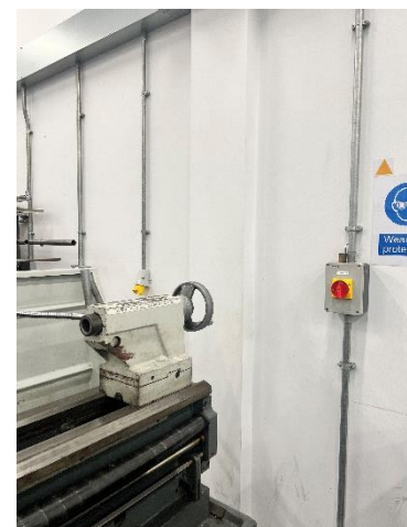
Figure 1.5 shows the centralisation tool as well as the lockable power switch and health and safety guidelines poster (Dunstan, 2024)
