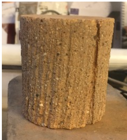
FIGURE 96 A CYLINDER OF BRICK CUT BY WATERJET AT UWTSD, EXHIBITS THE “DRAG” PHENOMENON
