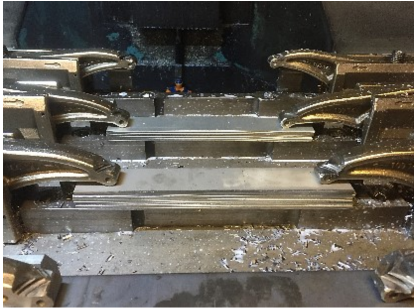
FIGURE 73 CURRENT CLAMPING SYSTEM FOR MILLING IN THE METALLURGICAL LABORATORY.
