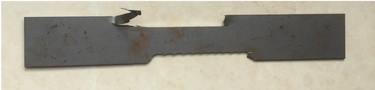
FIGURE 28 ATTEMPTED TENSILE SPECIMEN PRODUCED BY MILLING WITH NO PACKING MATERIALS AND A TOOL WORN TO ABOVE 5MM OF WEAR.
