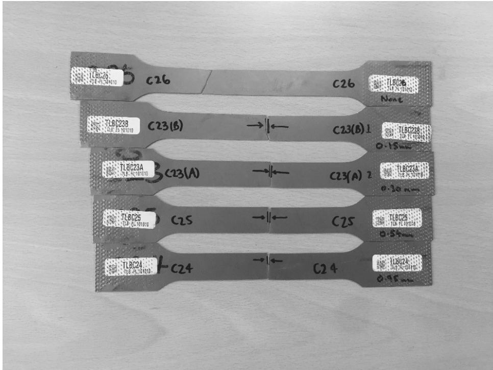
FIGURE 24 BROKEN SPECIMENS MARKING TEST FRACTURE AT THE POINT OF EACH NOTCH.
