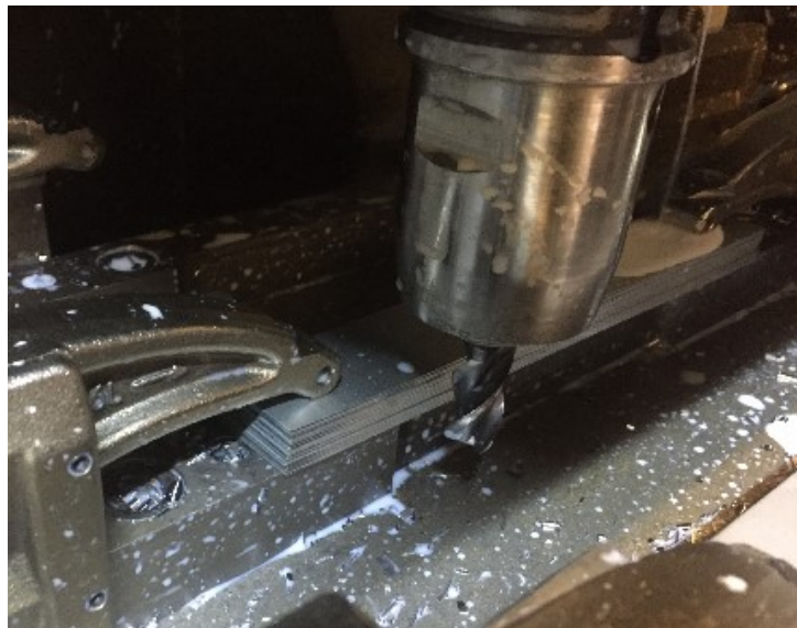
FIGURE 6 THE FINISHING TOOL FOR MACHINING TENSILE SPECIMENS AT THE METALLURGICAL LABORATORY SHOWING PERIPHERAL MILLING.
