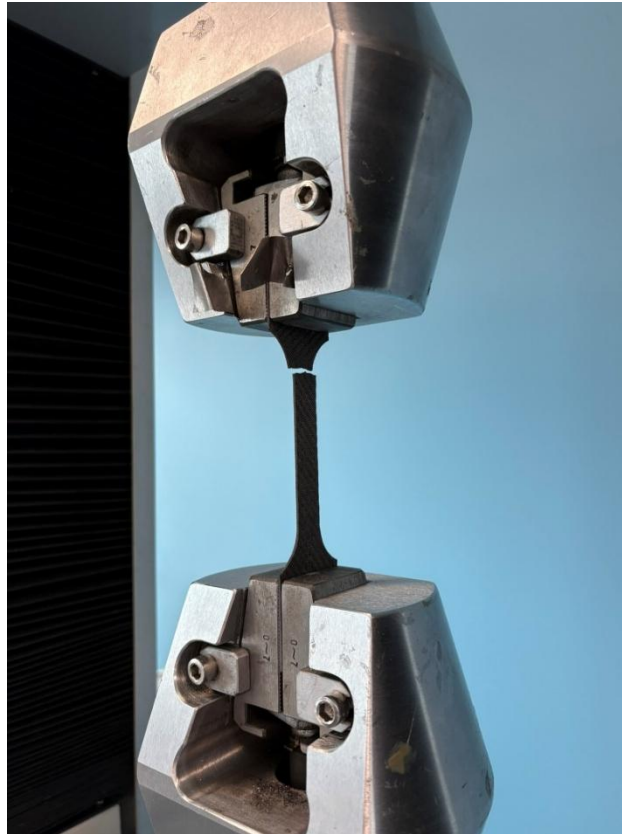
Figure 6 - Composite tensile specimen after failure in test grips.
