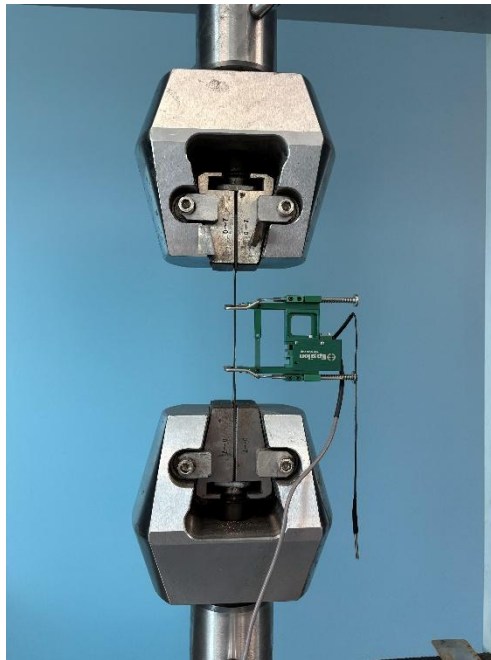
Figure 2 - The Denison tensile test machine with the extensometer fitted to a specimen.
