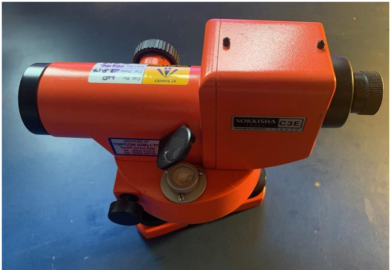
Typical Optical Level
