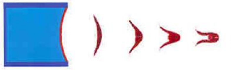
Figure 8-31 Computer model of an EFP dish forming a slug
