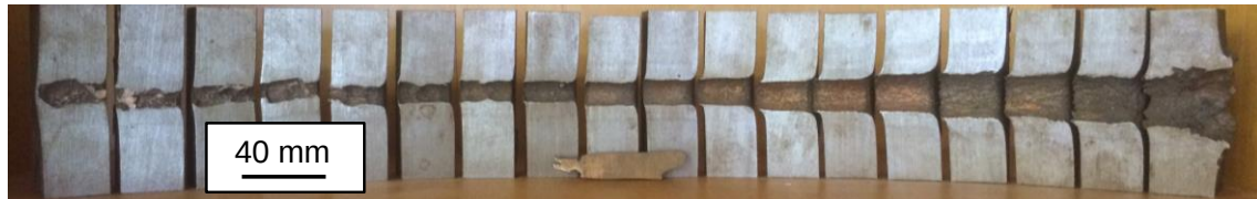
Figure 8-26 Photograph showing sectioned mild steel blocks penetrated by a small-scale shaped charge.
