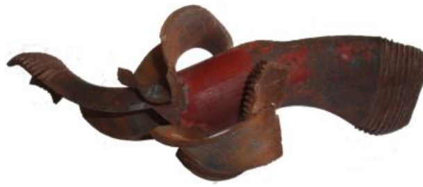
Figure 8-2 Metal tube following a deflagration type explosion
