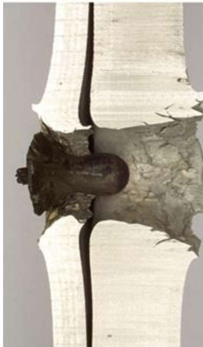
Figure 8-32 Recovered EFP projectile placed in a penetrated aluminium target
