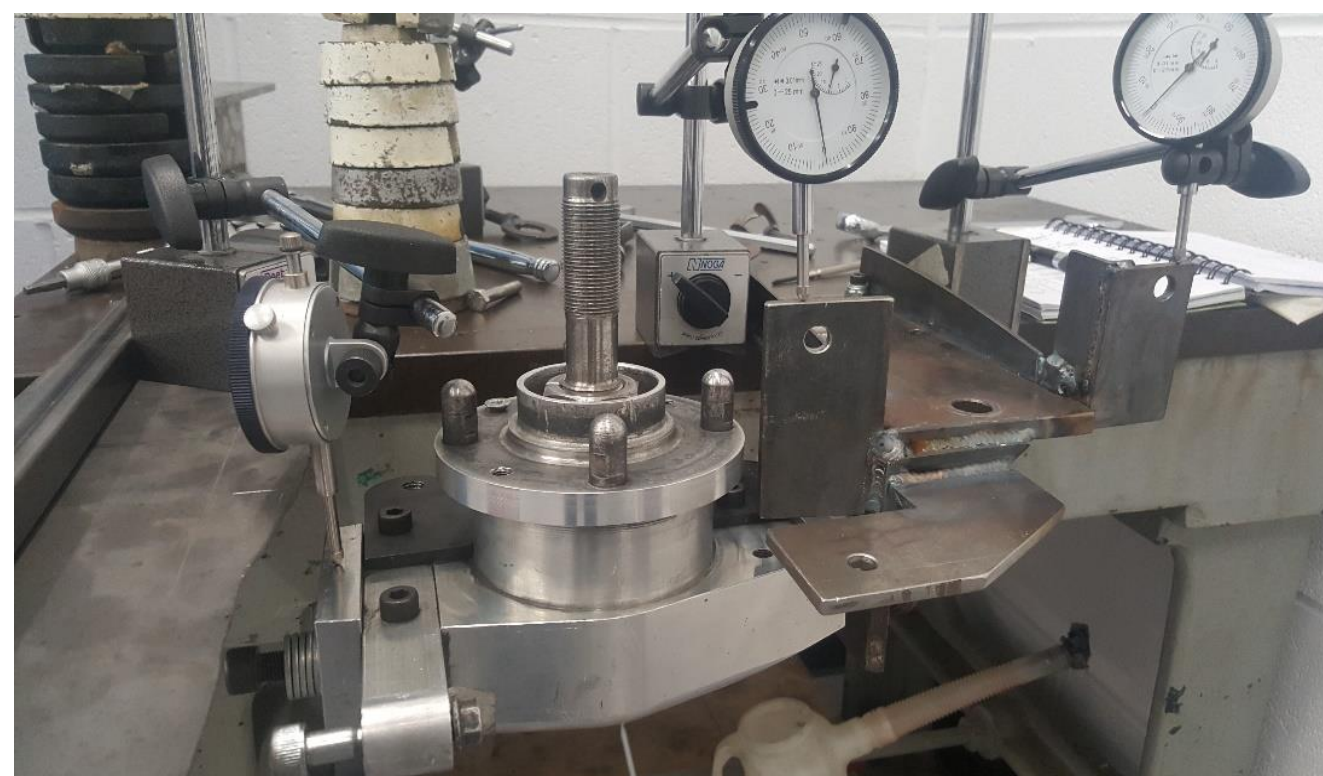
Workshop Test of Top Attachment Point in Y Direction.
