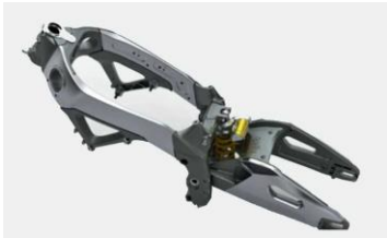
(Image 5A Perimeter/Twin Spar Frame).
