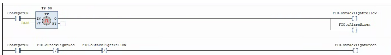
Figure 4-Codesys ladder logic for start-up and stack light sequence
