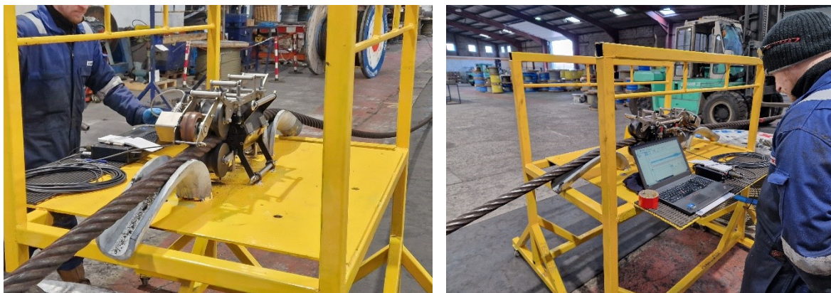
Figure 35 - MRT testing at the Certex facility
