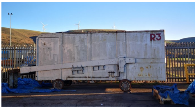
Figure 2 - Skip car for material hoisting and wire rope drum [2]
