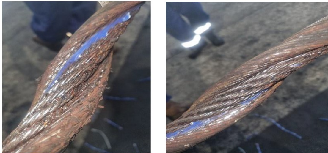
Figure 41 - Wire rope one and two showing internal corrosion at 55m and 53m
