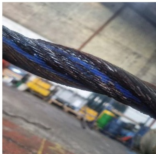
Figure 40 - Destructive testing of the wire rope at 42m
