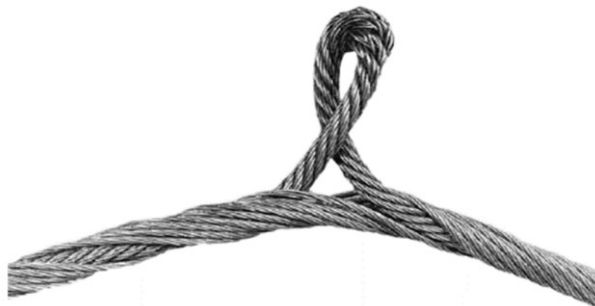
Figure 22 - Example of core protrusion due to torsional effects [32]
