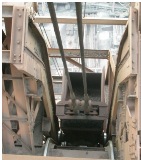
Figure 3 - Skip car terminations and compensation arm
