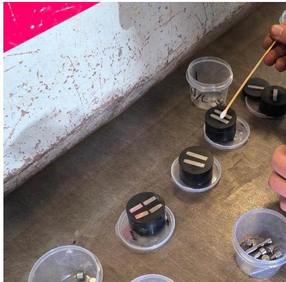
Figure 23-Application of 5% Nital to etch the surface of microscopy samples.
