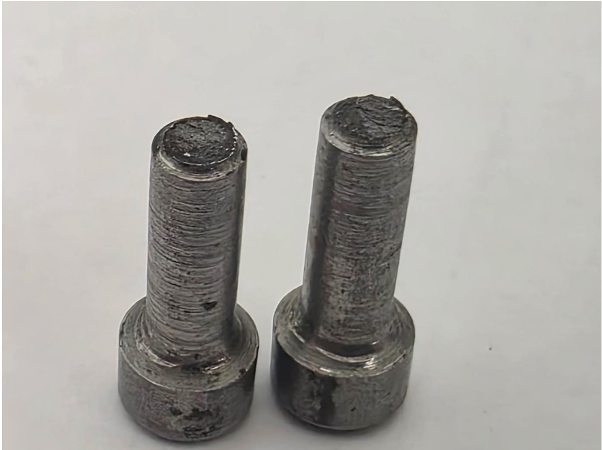
Figure 40-3.2 \mu m notched specimens showing minimal plastic deformation.
