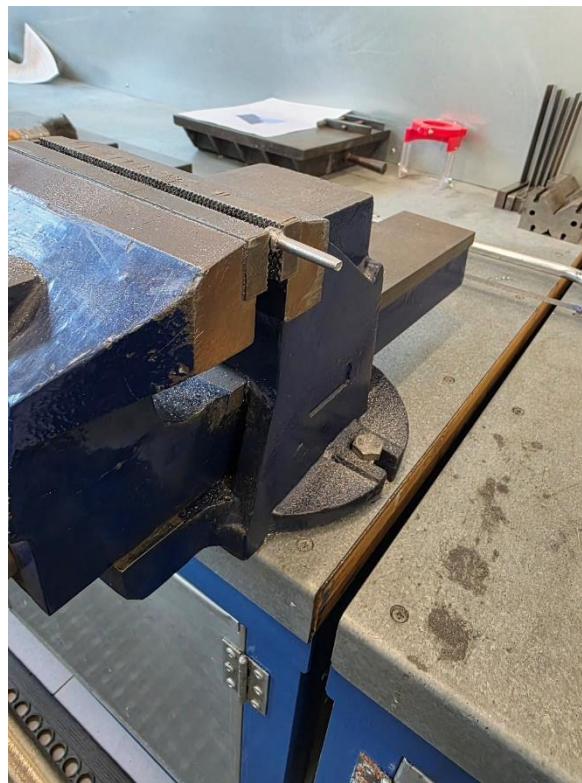
Figure 19-Sample mounted in bench vice in preparation of filing.
