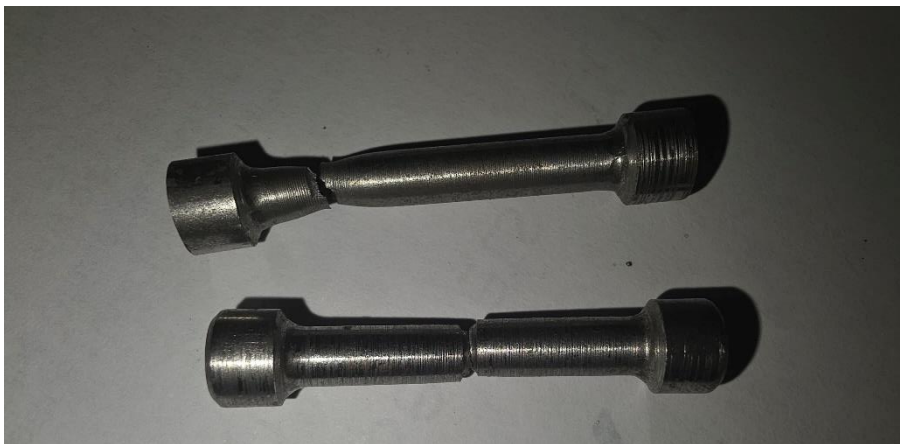
Figure 41-A side-by-side comparison of conventional ductile failure with the failed notch specimens.
