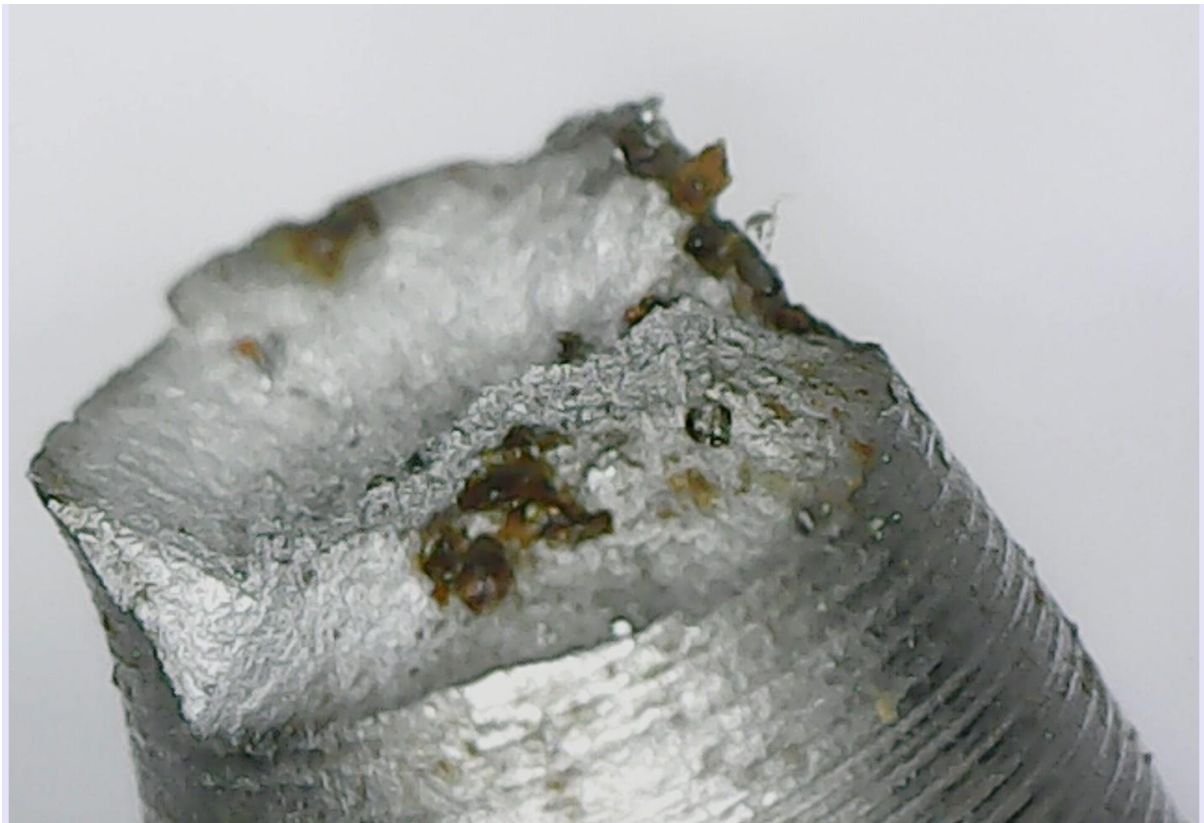
Figure 37-Image depicting the ductile failure mode of a 1.6 \mu m specimen (with coolant).
