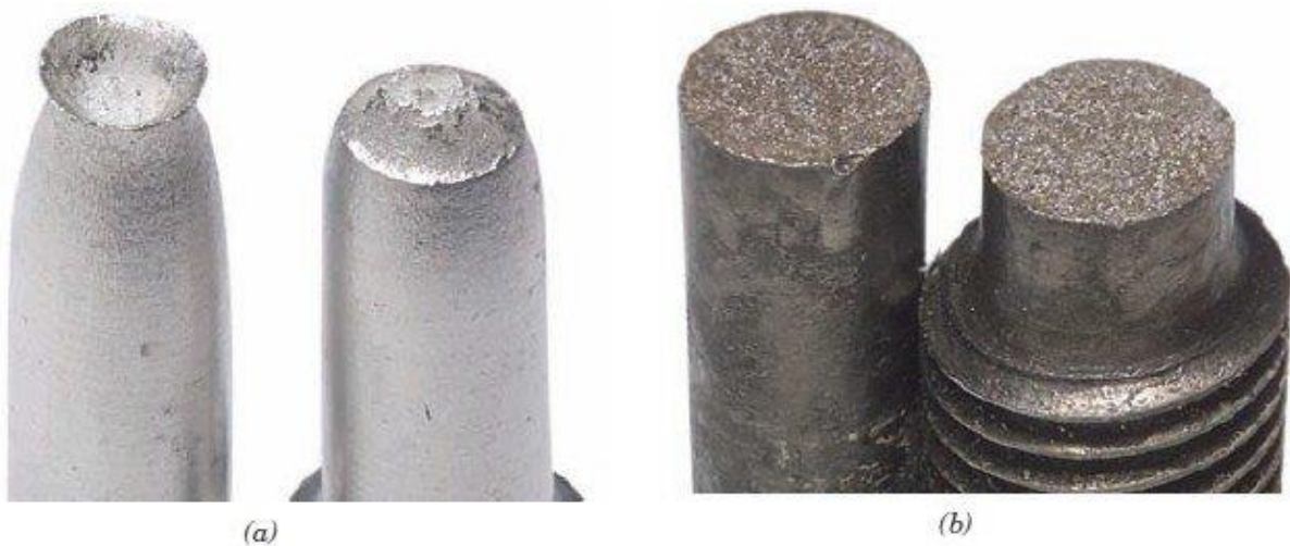
Figure 9-Examples of (a)ductile and (b) brittle failure. Source:(Callister and Rethwisch, 2020)
