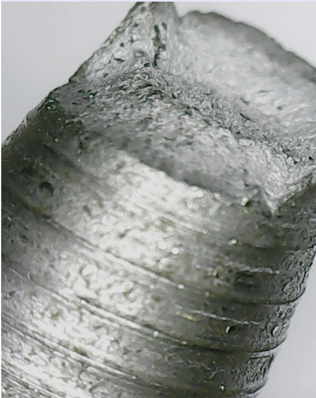
Figure 35-Image depicting the ductile failure mode of the 6.4 \mu m specimen.
