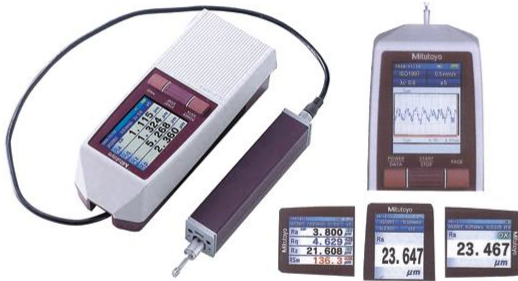
Figure 13-Mitutoyo Surftest surface profilometer. Source:(Surface Roughness Measuring Systems | Mitutoyo America Corporation, 2025)
