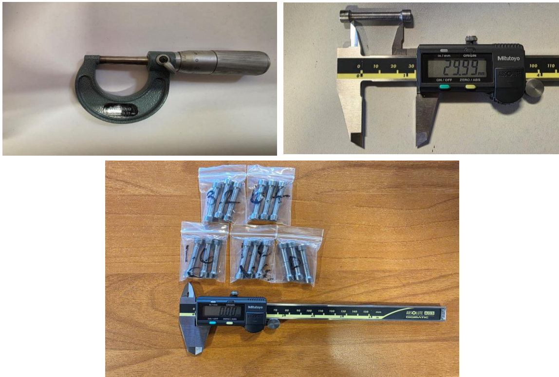
Figure 12-0 to 25mm Mitutoyo micrometer and 0-150 Mitutoyo digital vernier with test specimens
