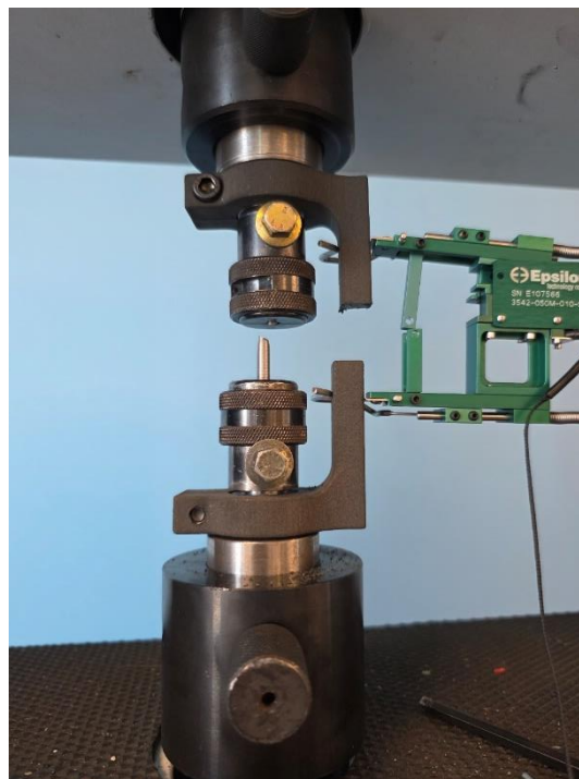
Figure 17-Fractured test specimen post-test.
