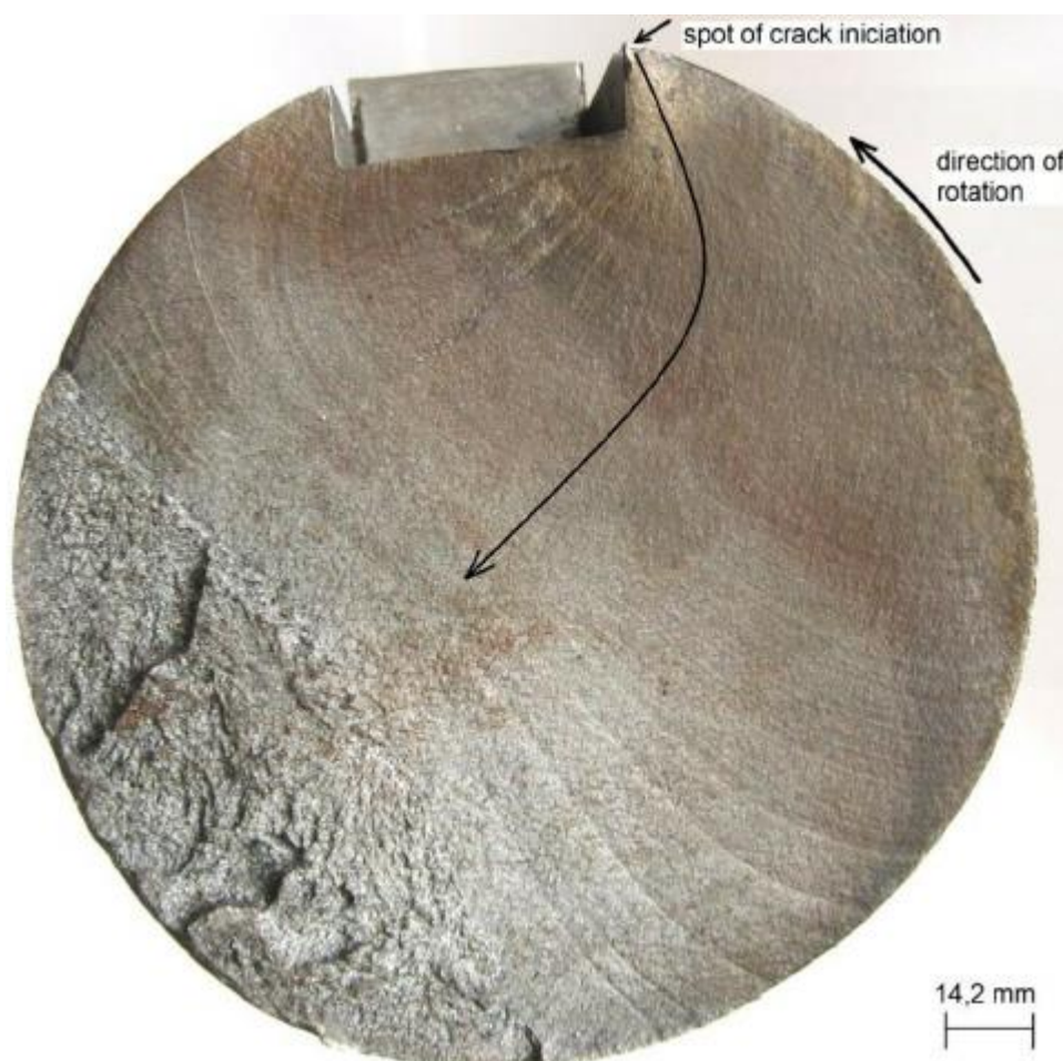
Figure 8-Image depicting crack initiation from a keyway. Source:(How does a propeller 'fall off'? - Professional Mariner Forum, 2020)
