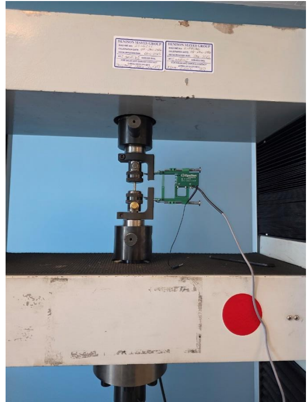
Figure 15-Test specimen mounted in the split collar and assembled fully with the extensometer.
