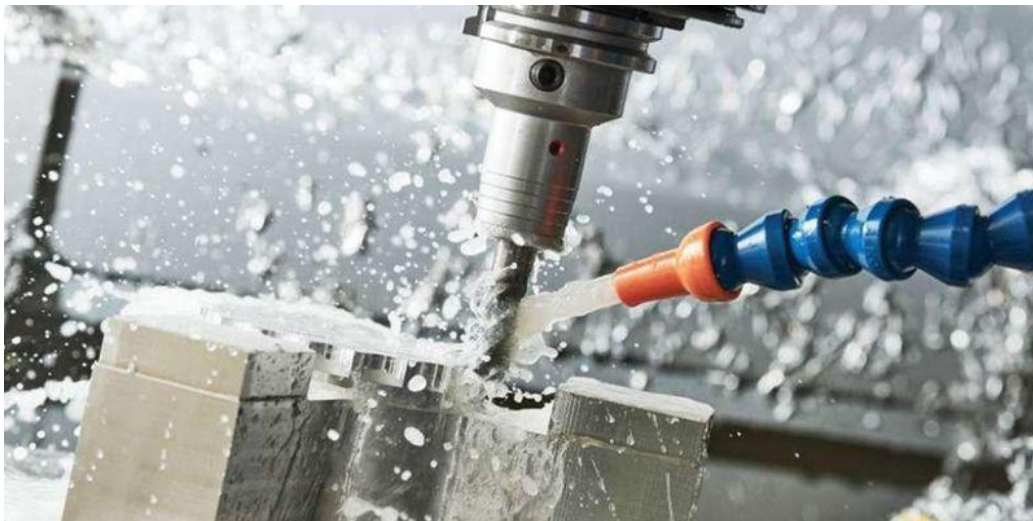
Figure 7-Image of a milling machine using soluble oil coolant. ('Types of CNC Coolants: How to Choose One in Machining?' - WayKen', 2023)
