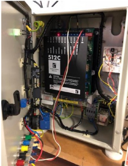
Figure 26: Parker 512C motor drive
