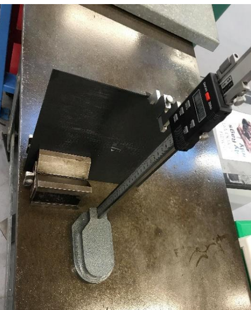
Figure 1: Photo of the measurement process used when recording the dimensions of the carbon fibre before and after the test sample has been exposed to heat (Lillicrap, 2019)
