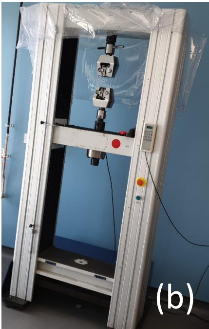
Figure 2: (a) Test Samples with Thermocouples Attached in Autoclave for the thermal cycling tests. (b) Denison Tensile Machine used for Tensile Testing
