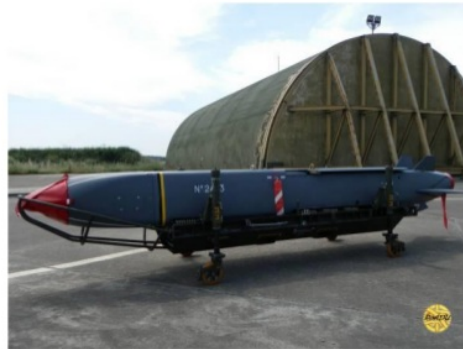
FIGURE 16 airfield/ maintenance general handling missile handling dolly
