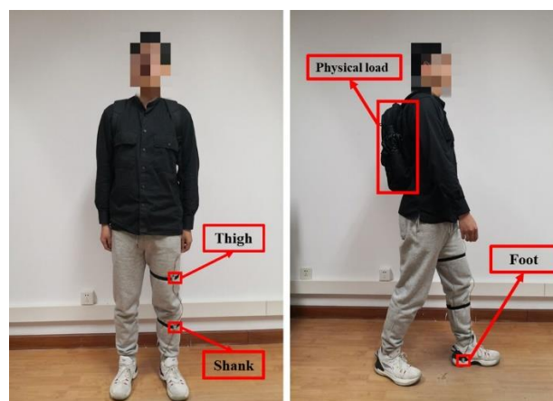
Figure 10 IMU sensor markers for lower limb fixation and backpack weighting
