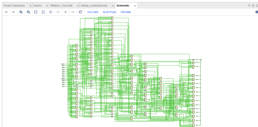
Figure 29 - 8x8 Wallace Tree Multiplier Implementation Schematic
