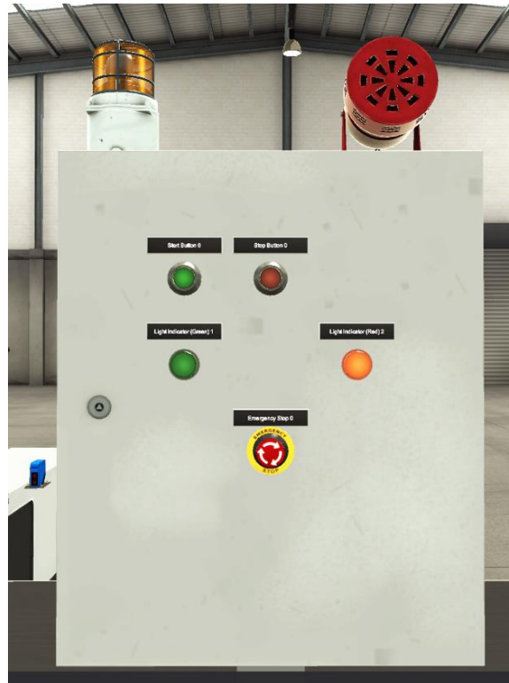
Figure 25 - Control Panel with indicators and buttons
