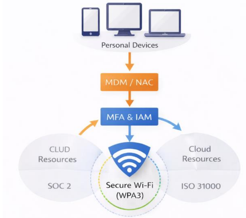
Figure 4:BYOD and Wireless Security Control Architecture
