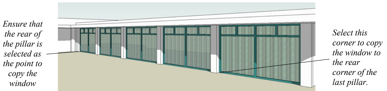
Figure 56. The completed window internally arrayed along Building 1.
