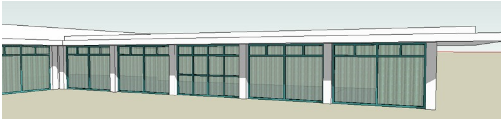
Figure 58. The middle bay of Building 1 altered to include doors
