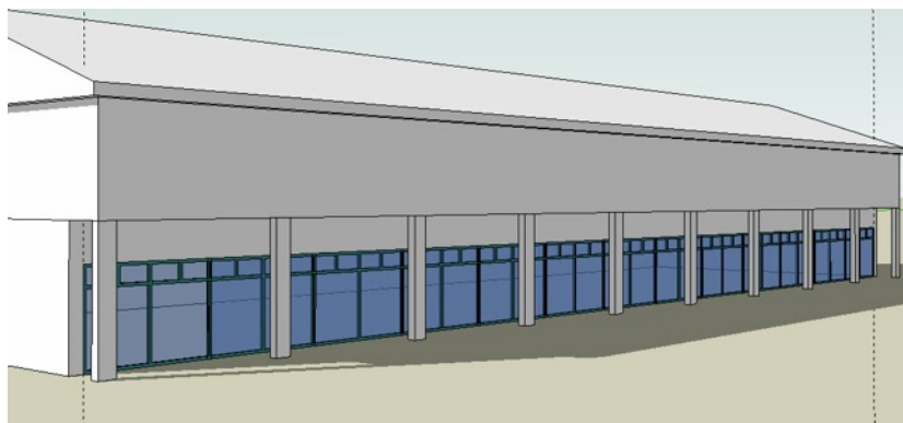
Figure 61. Ground floor window6 component copied and arrayed
