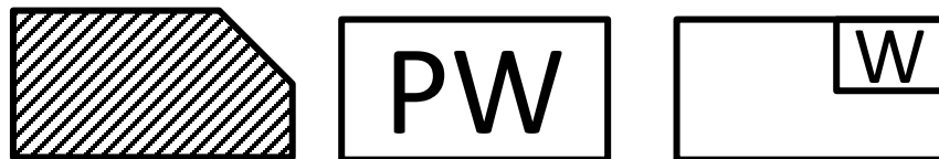
Withdrawal Kanban (and alternative)
