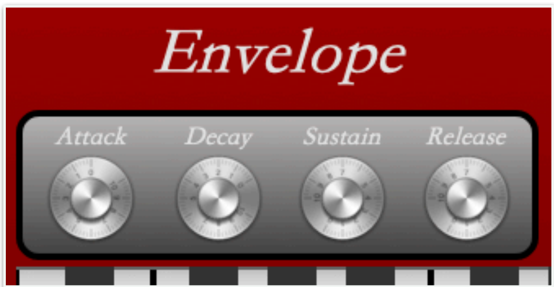
Fig. 13 HISE: ADSR Panel controlling the envelope of the sound.
