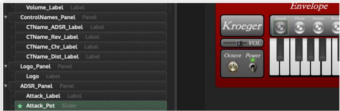
Fig. 3 HISE: Attack knob selected in the interface designer window on the right (green box) and highlighted on the left (in green) where the option to duplicate it was not working.
