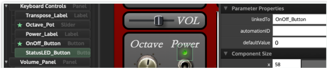
Fig. 14 HISE: Highlighted Status LED Button in the component list. Highlighted panel in GUI designer (centre). Parameter Properties showing linkedto: OnOff_Button (right).
