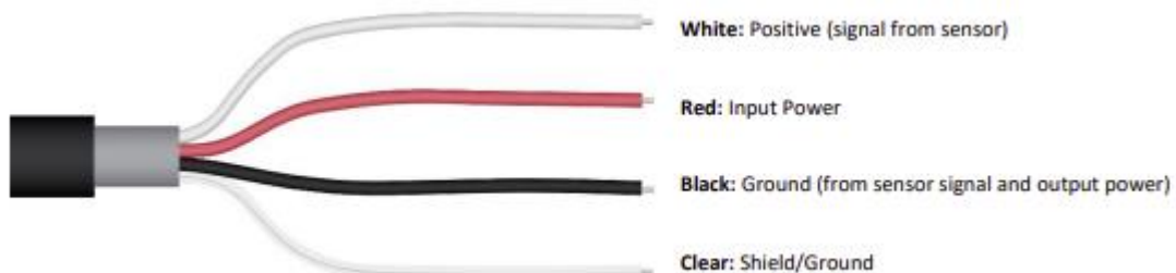
[56] Figure 40 - Apogee Instruments SU-202-SS UV Sensor Wiring
