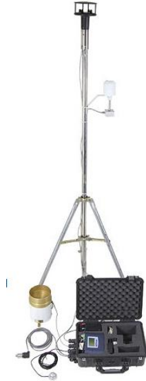
[8] Figure 6 - RWS-07 Portable Weather Station
