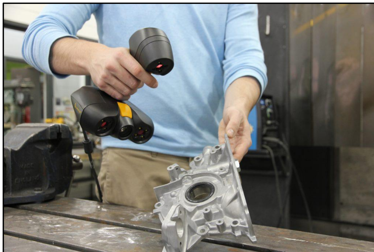
Figure 5: 3D scanner Peel-3d (capture-point. [Online])
