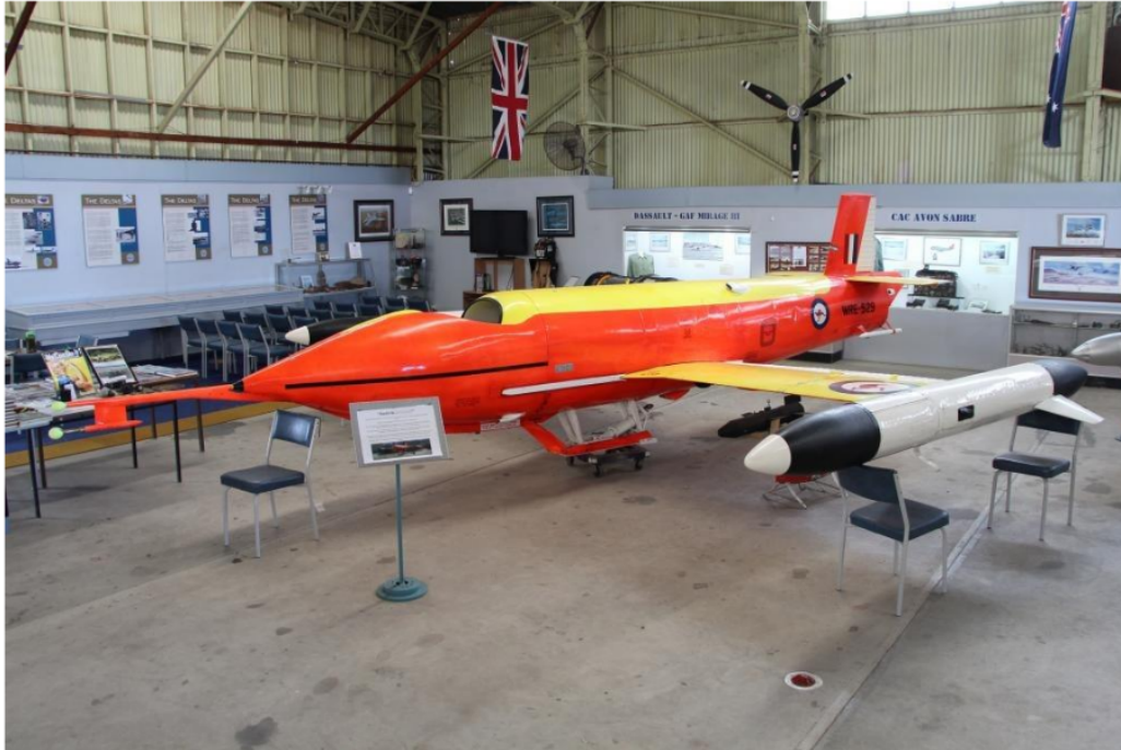
Figure 2-2- Mid 1900 aerial target system (Jindivik) [17]
