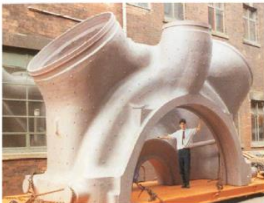
Steel casing for a nuclear power plant (courtesy of Sheffield Forgemasters Engineering Ltd.)
