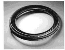
Picture: A one-piece compressor stator with 108 separate airfoils made by investment casting (photo courtesy of Howmet Corporation)
