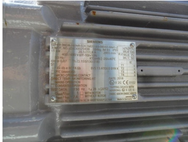
Figure 12 - Motor details plate
