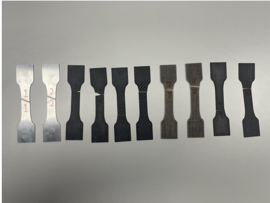
Figure 3: Two specimens of each material after testing to failure. Note that aluminium split in the centre whereas the composite materials broke at the end of a radius, which acts as a stress concentrator.
