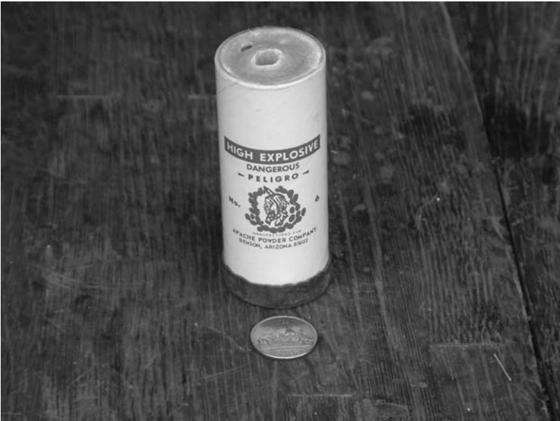
Figure B.13 Cast booster.
