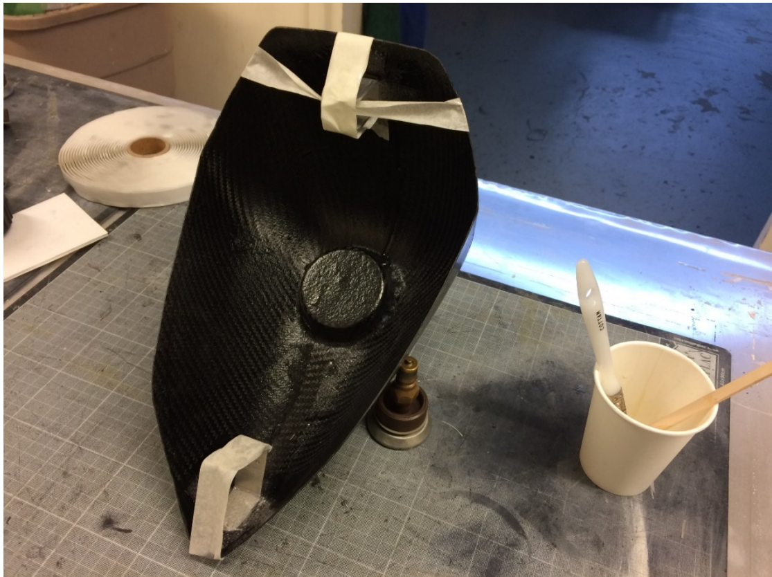
Figure 33 – Bonding of brackets with fibreglass and resin (Przibylla, 2017/2018)
