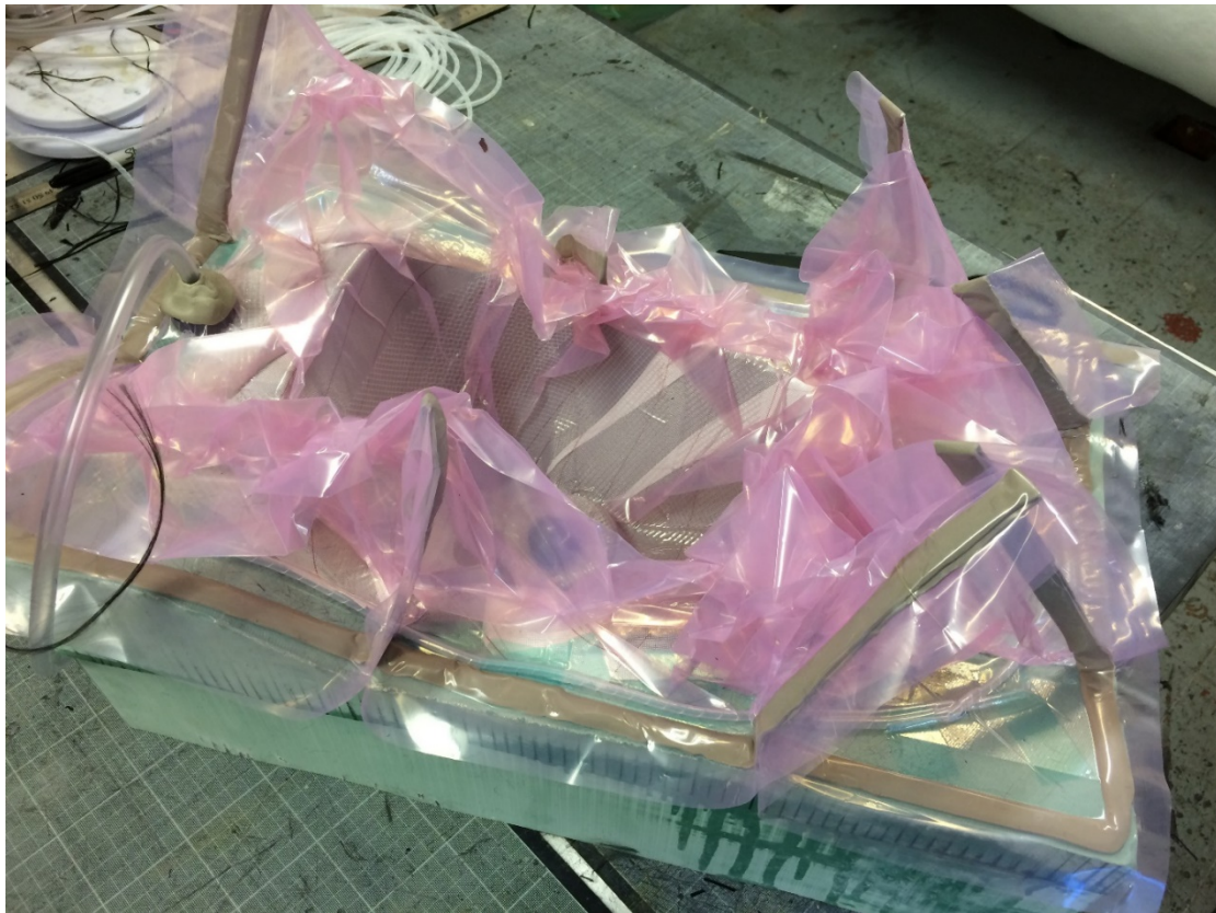
Figure 29 – Vacuumed and sealed mould with the carbon fibre part (Przibylla, 2017/2018)
