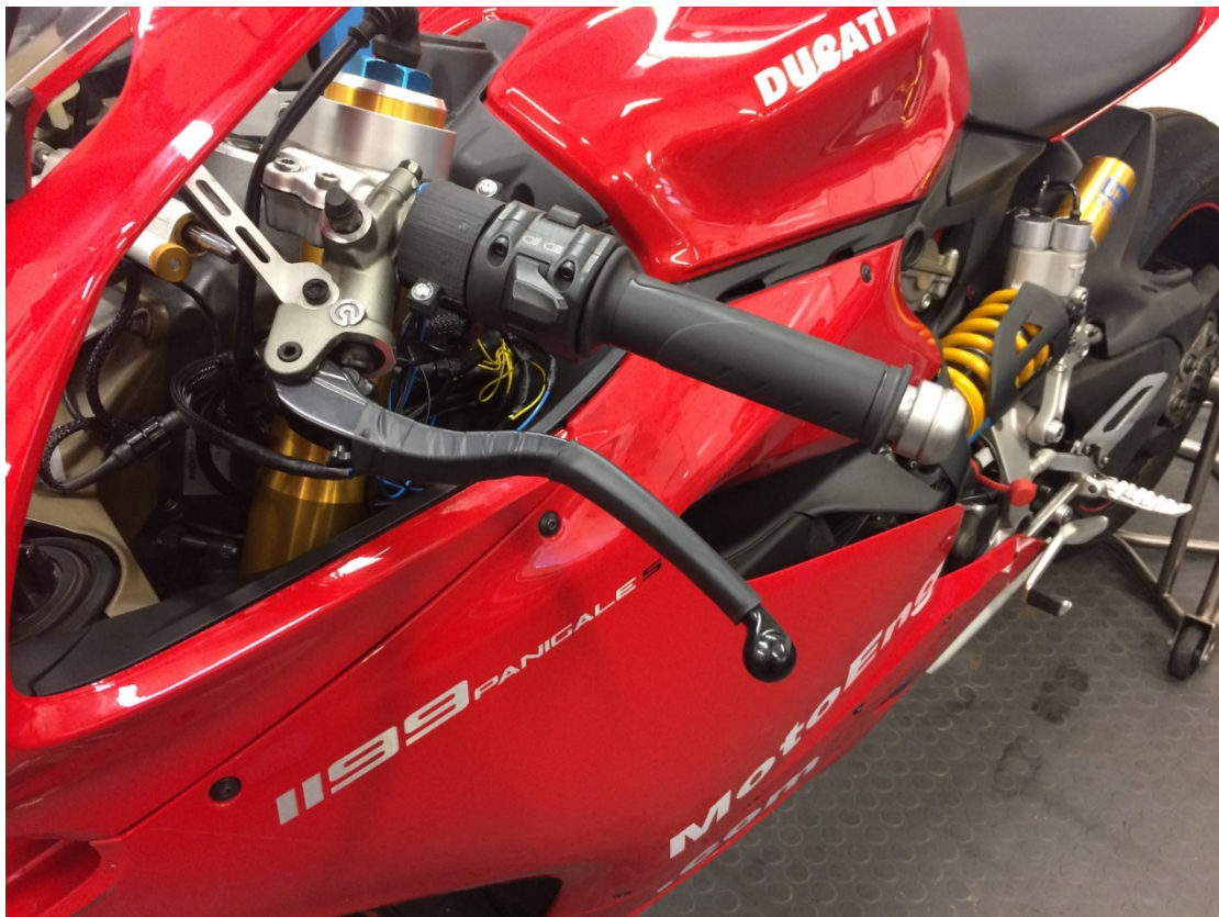
Figure 16 – FSLP fitted to the clutch lever on the left handlebar tube (Przibylla, 2017/2018)
