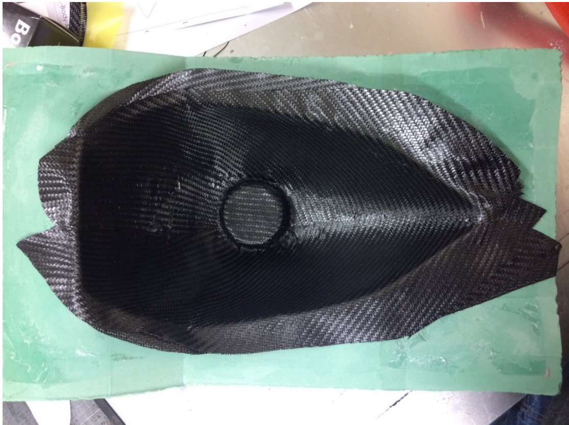
Figure 30 – Pre-impregnated carbon fibre layers inside the mould (Przibylla, 2017/2018)
