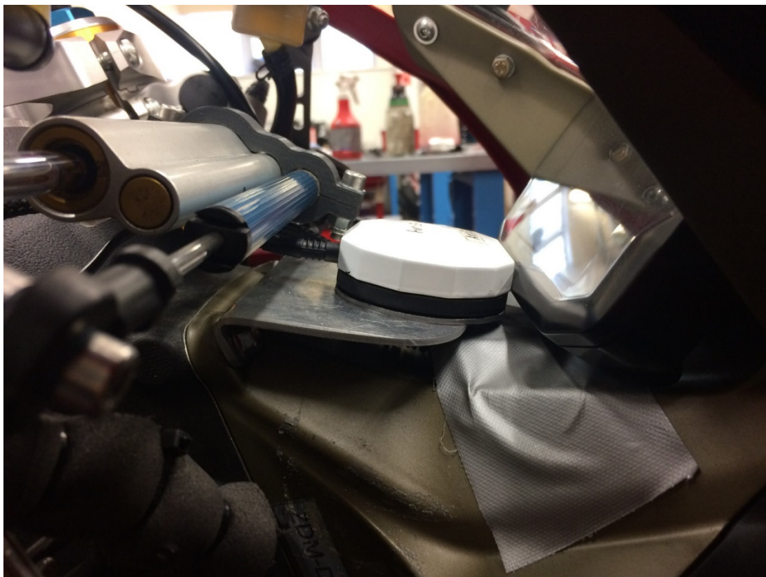
Figure 35 – GPS antenna on a custom-made bracket that is mounted to the front of the chassis (Przibylla, 2017/2018)
