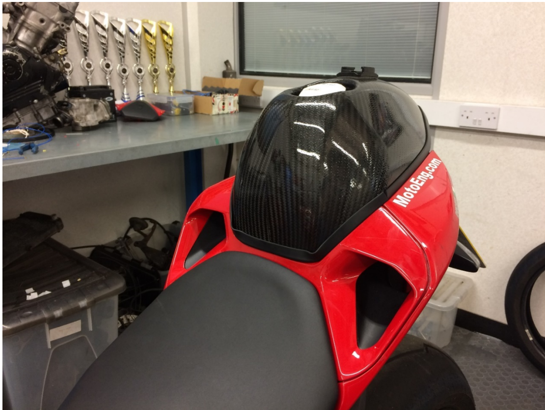
Figure 38 – Finished seat unit cover and data acquisition setup (Przibylla, 2017/2018)
