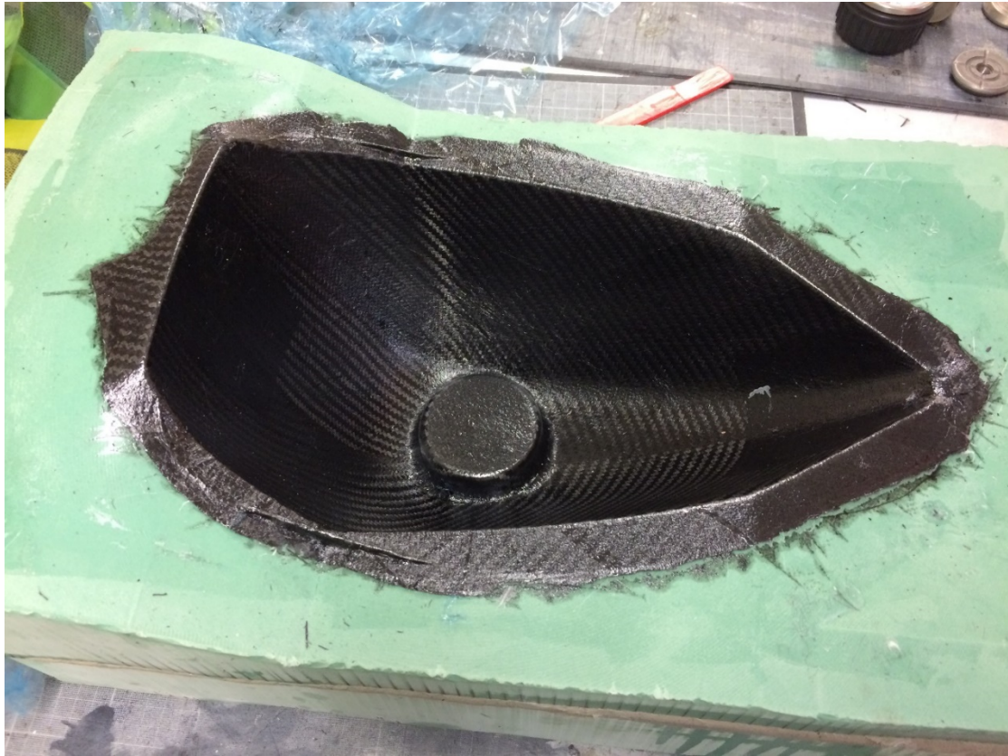
Figure 32 – The carbon fibre seat unit cover after curing in the autoclave (Przibylla, 2017/2018)
