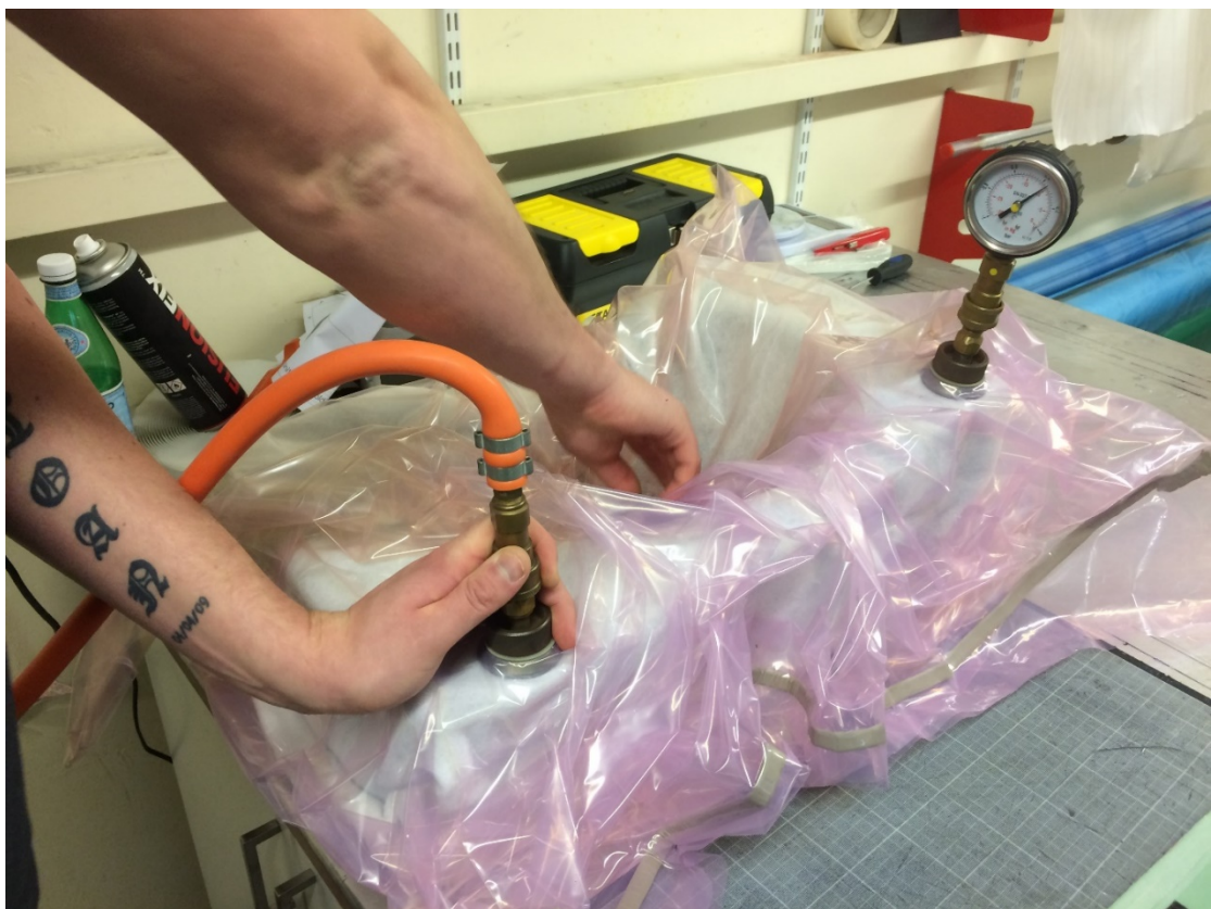
Figure 31 – Bagging and vacuuming as preparation for the autoclave (Przibylla, 2017/2018)
