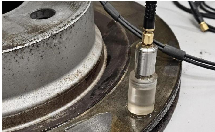
Figure 26 - UT Probe with a block affixed
