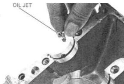
Figure 3- Oil Jet Location (Honda, 2006, p. 192)
