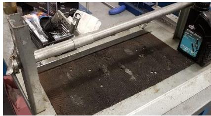
Figure 6- Homemade Spring Compressor Tool (Sorg, 2018)
