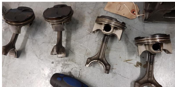
Figure 5-Pistons Removed and Numbered (Sorg, 2017)
