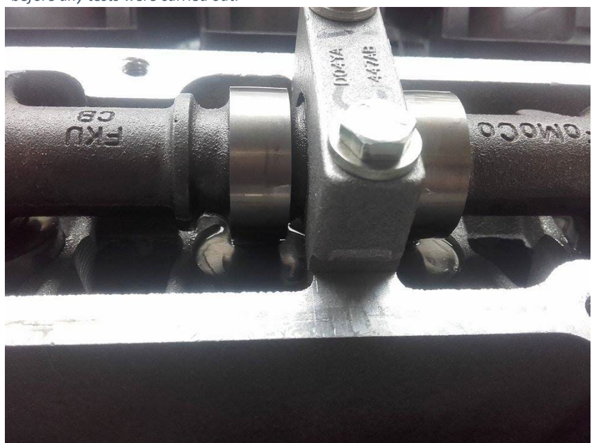
5 Photo of the Inlet Cam in place in the engine. The lobes were Pre oiled before any tests were carried out.
