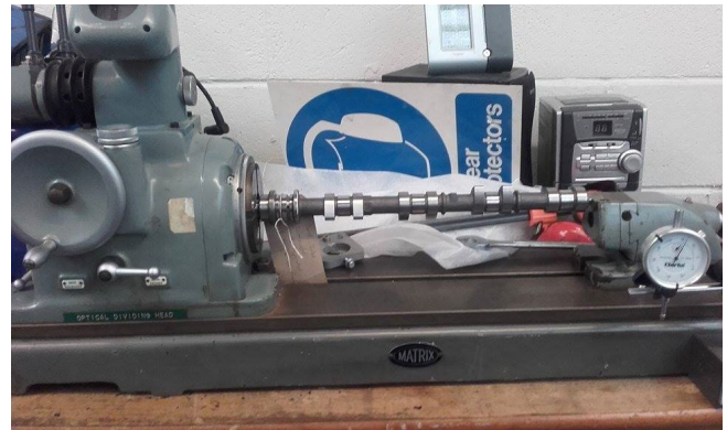
Fig.6: Measuring Camshaft Shape
