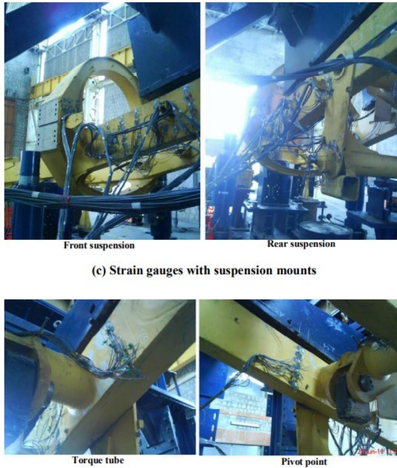
Figure 4 Strain Gauges Fitted to Critical Areas (Dhandapani, 2012)
