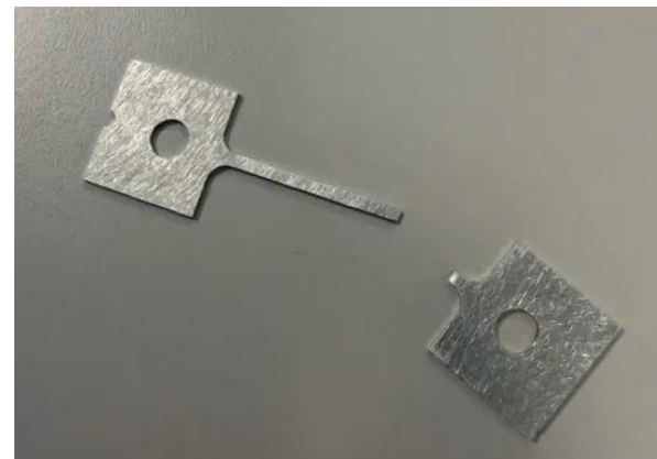
Figure 3 Aluminium Specimen after fracture
