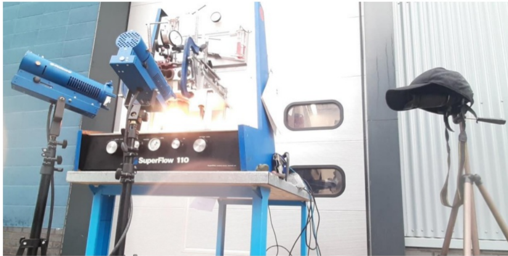
Figure 5-6: In-Cylinder Turbulence Visualization Experiment Setup
