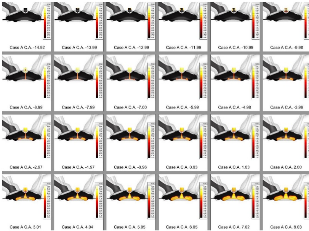
Figure 6-7: Case A Temperature Contour Side View
