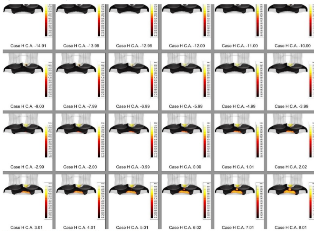
Figure 6-27: Case H Temperature Contour Front View
