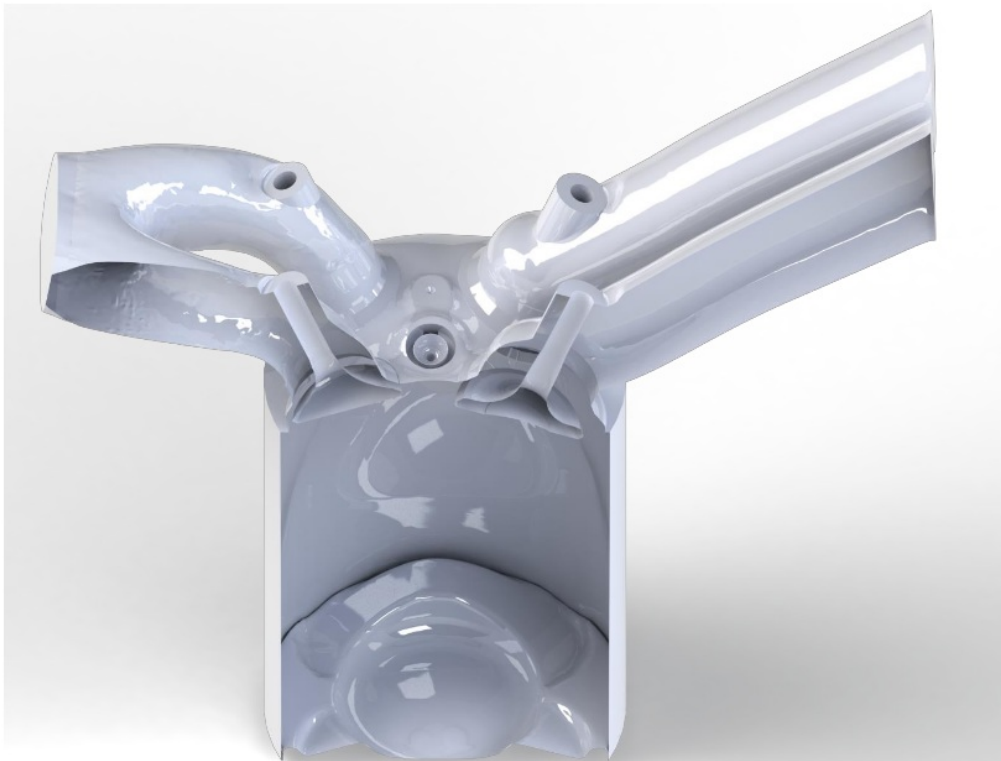
Figure 5-1: Rendering of the Finished Ford Fox GTDI Surface Assembly
