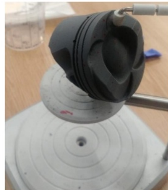
Figure 9-60: Piston Crown of the Ford Fox GTDI Engine in the Process of Surface Scanning
