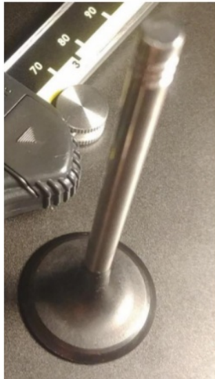
Figure 4-13: Exhaust Valve of The Ford Fox ICE
