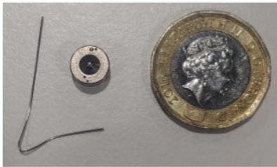
Figure 9-63: Scale of the BOSCH Direct Fuel Injector Tip from Ford Fox GTDI Engine
