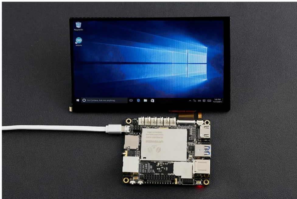
Figure 9.1: LattePanda Board running Windows 10 with 7" screen
