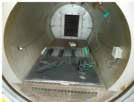
Figure 19: Test Samples in the Autoclave with Thermocouple Attached (Lillicrap, 2019)
