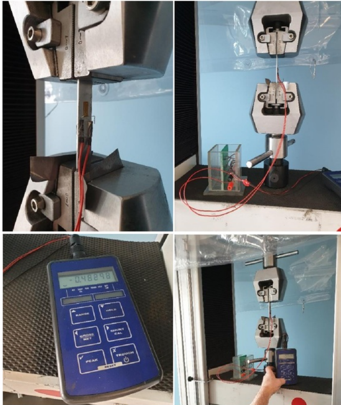
Figure 30: Strain Gauge Attached to Test Sample (Lillicrap, 2019)
