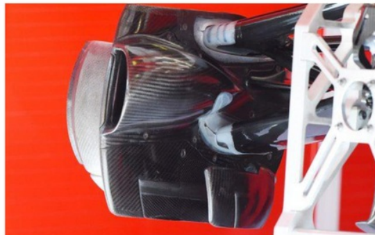
Figure 5: Carbon Fibre Brake Duct (Formula1.com, 2018)
