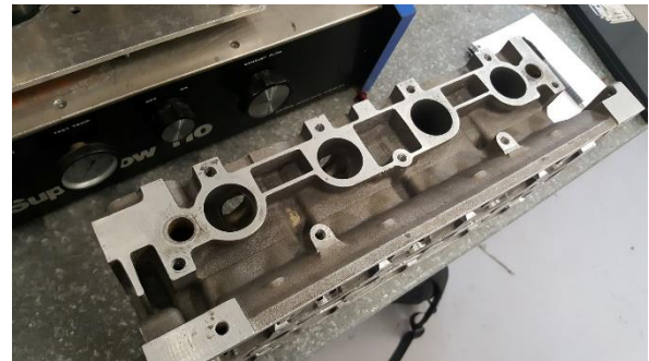
Figure 14 - Modified cylinder head (intake side). (Kot, 2018)
