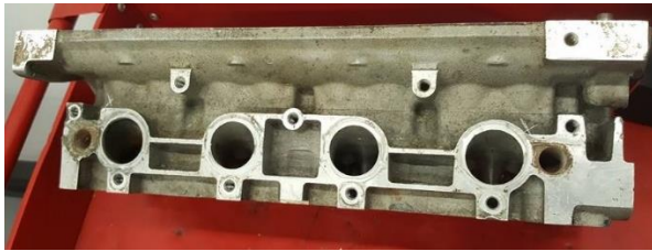
Figure 13 - Standard cylinder head (intake side). (Kot, 2018)
