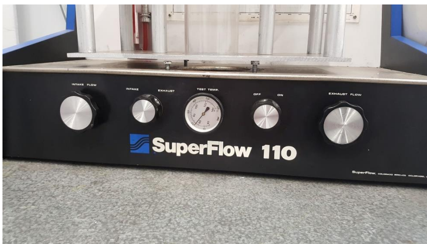
Figure 3 - Flow bench controls. (Kot, 2018)
