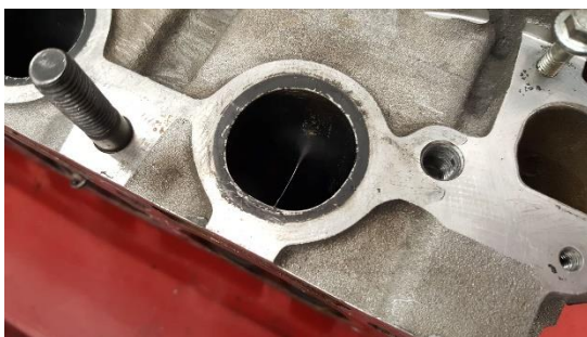
Figure 12 - Modified exhaust port. (Kot, 2018)
