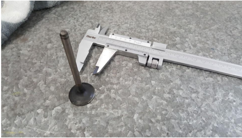
Figure 2 - A valve being measured with a vernier caliper. (Kot, 2018)
