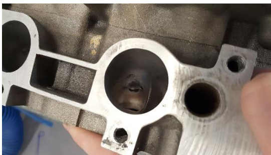
Figure 10 - Modified intake port. (Kot, 2018)
