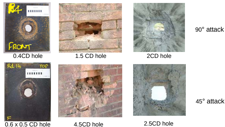
Figure 2; Armour and structure targets defeated by copper lined SSJ warhead
