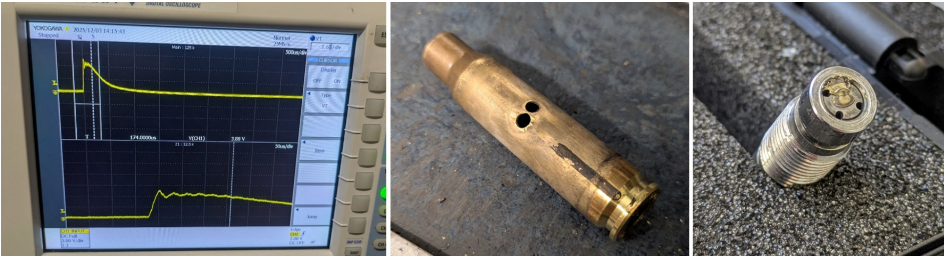
Strike! The consequences of case misalignment. The £4,000 transducer saved by the £80 "diaphragm protector"
