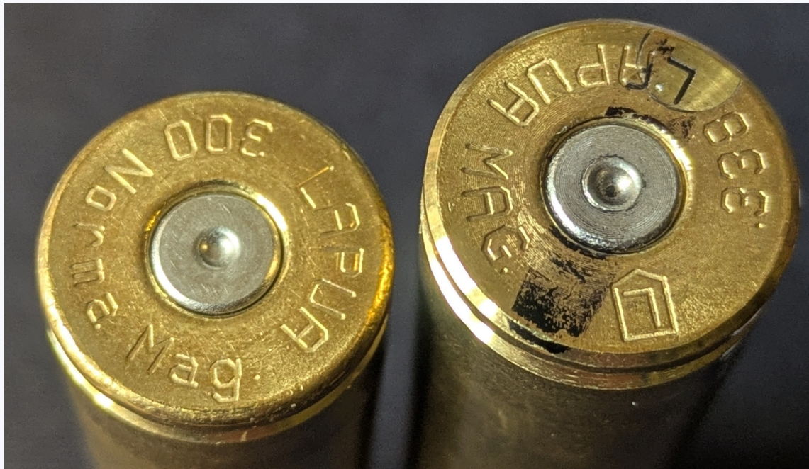
Normal & excess pressure signs
