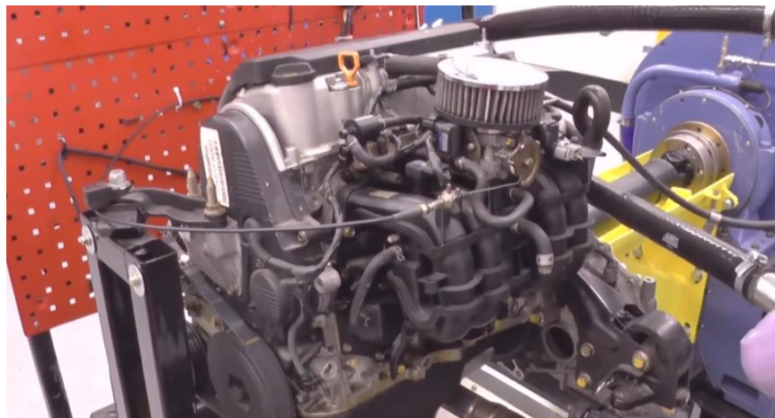
1 Figure 1 Image of Honda D16 VTEC Engine connected to Dynamometer (UWTSD, 2020)
